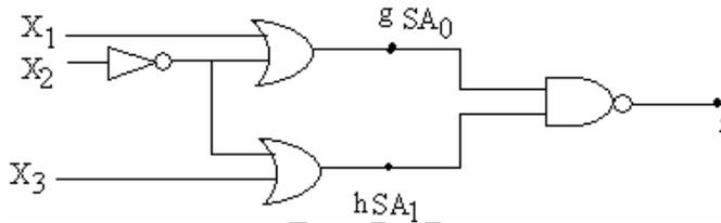
8. Design a test pattern generation to test the following sequential unit. [16]
